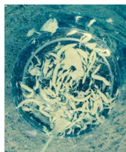
Incompatible mix of UNIFORM plus Liquid NP.
